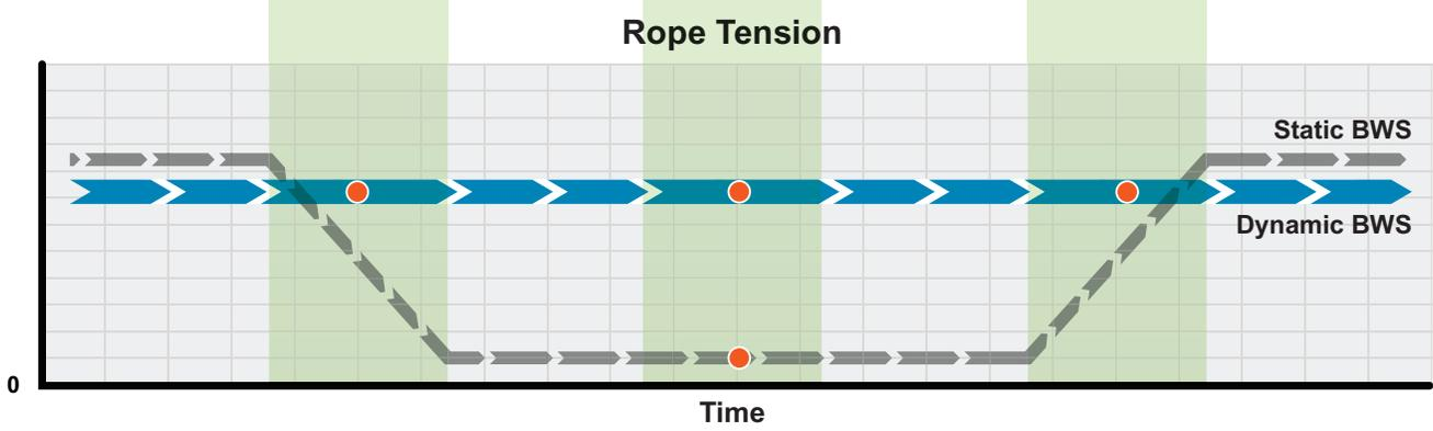
During a step, Dynamic Body Weight Support keeps the rope taught in order to provide the selected unloading. This also prevents falls. Static Body Weight Support systems provide no such benefits during active movement.
