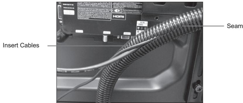
Figure 11: Inserting Cables into the Wire Loom
