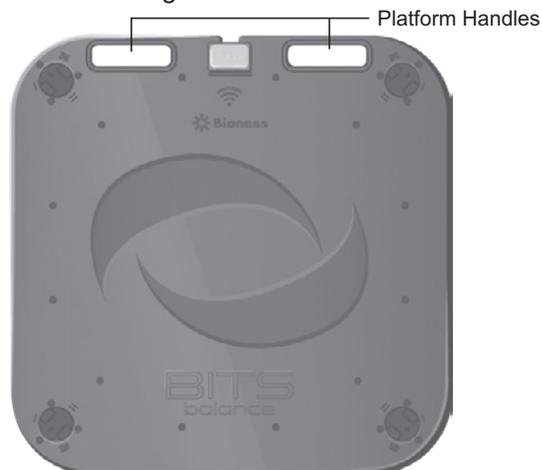
Figure 19: Handles for moving the Platform
