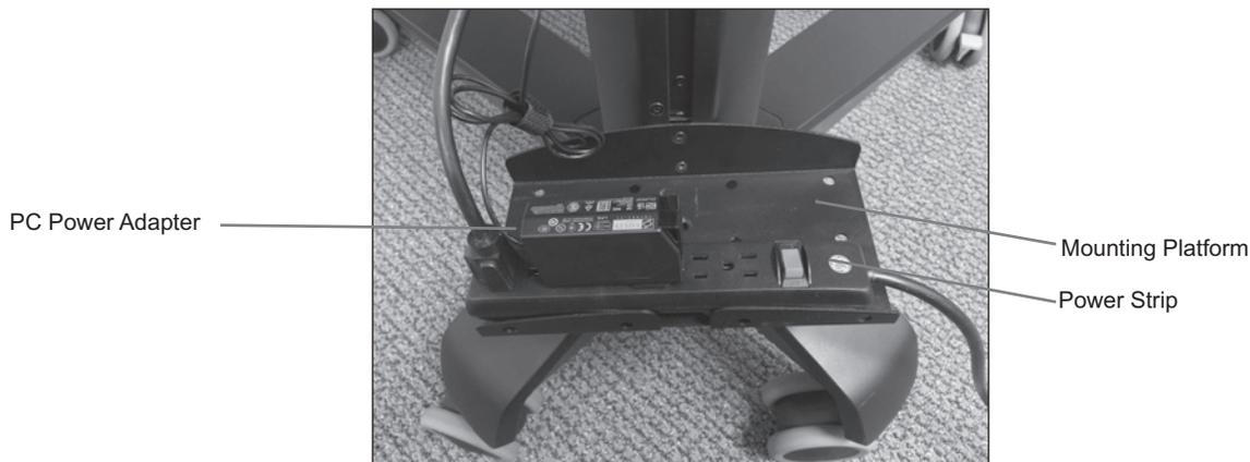
Figure 10: Mounted PC Power Adapter and Power Strip
